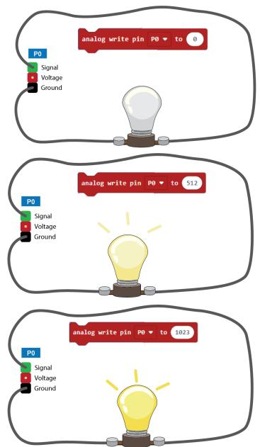
Note that the Microbit cannot create a true voltage change. It can only simulate it by rapidly switching the current on and off. This is called Pulse Width Modulation (PWM).
