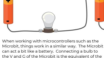
battery + and -, so the bulb lights up. But if you connect the bulb to the S and G instead,
