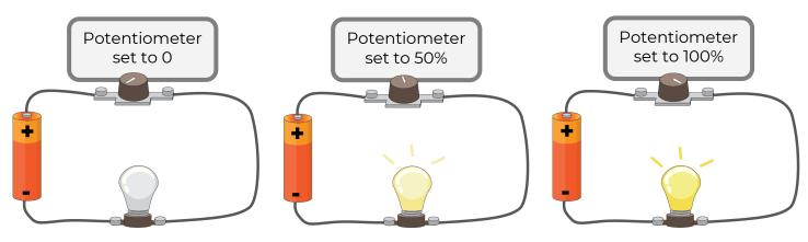
With the bulb connected to the S and G of the Microbit we can write an analogue value to the pin to give the effect of changing the voltage. You can write any value from 0 to 1023. A value of 0 means the pin is fully off. A value of 1023 means it is fully on. Values in between 0 and 1023 will give varying intensity.
