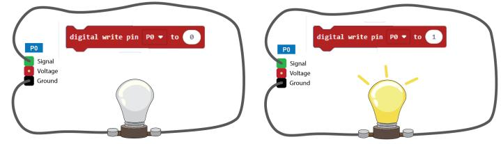
In this case we have a **digital output**. Digital means the output is either fully on or fully off.
