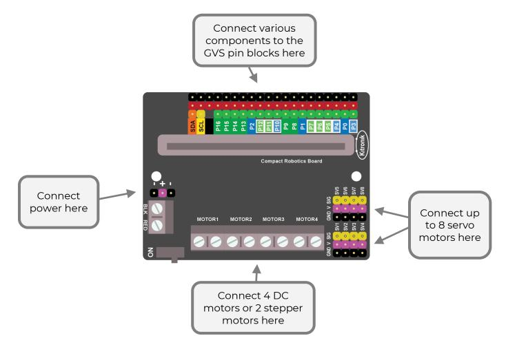
The motor controller board allows you to build robots, machines and lots of different motorised projects!
